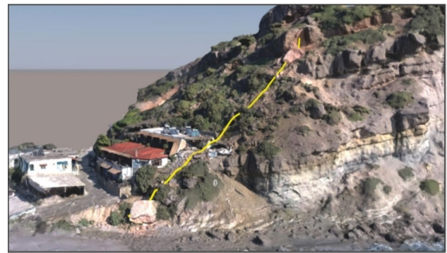
Fig. 11 Oblique view of the closest rockfall trajectory obtained from RocFall3 back-calculations superimposed on the 3D digital model
