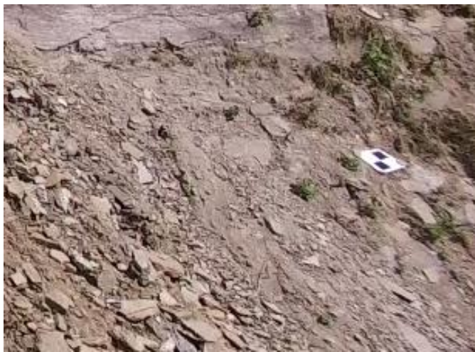
Fig. 3. Example of deployed GCP target.
