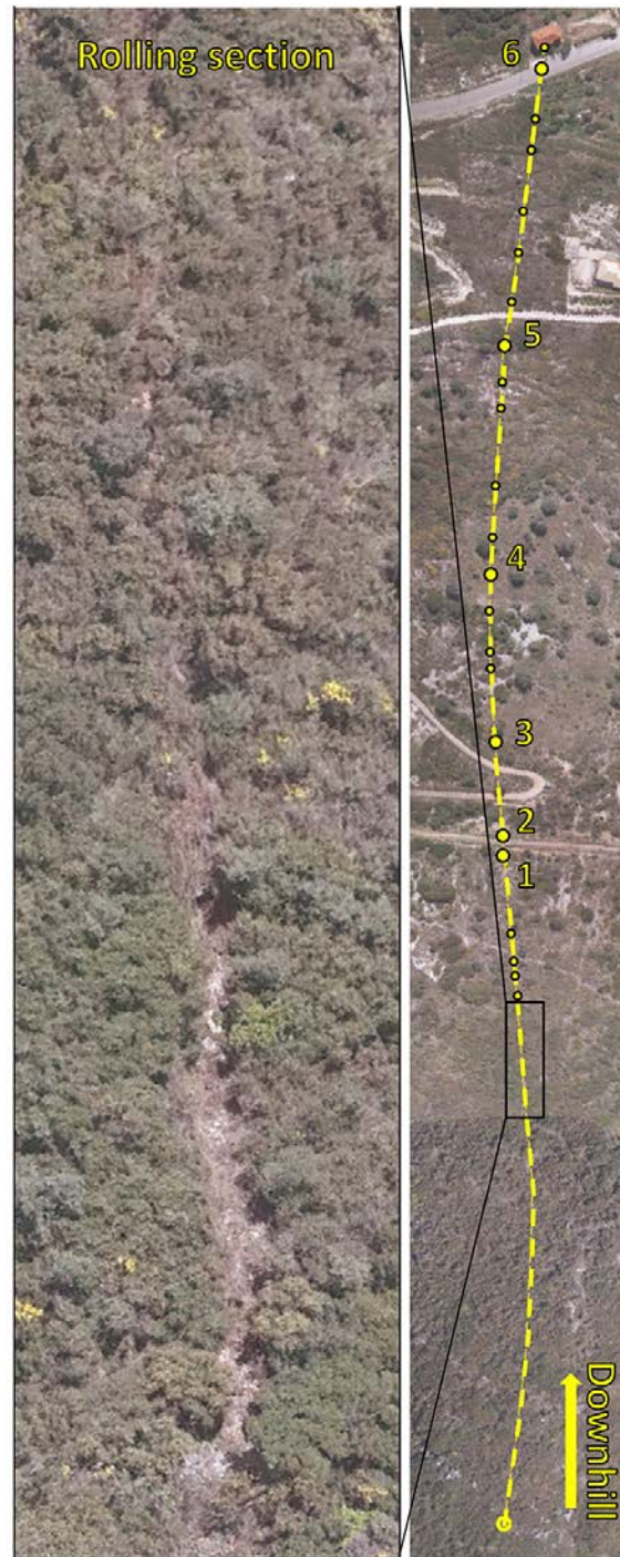
Figure 5. Top view orthophoto – Rolling section and bouncing positions recognition for the Ponti (Lefkada) rockfall.
