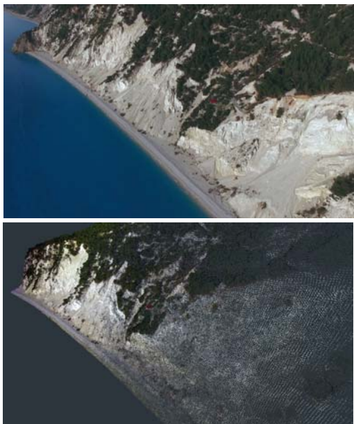
Figure 7. UAV-based 2D imagery (top) and 3D point cloud geometry (bottom) for an example site in Lefkada
