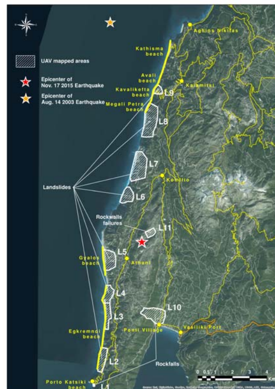
Figure 2. View of landslide affected areas mapped by Unmanned Aerial Vehicles (UAVs) in April 2016.
